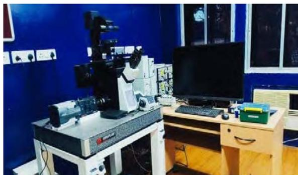
**Image 1: Newly installed Total internal reflection fluorescence microscope (TIRFM) at CRF(LSD).**
